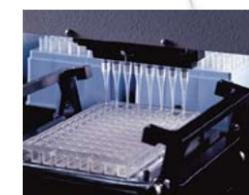
**8-channel pipettor accessing a 96-well microplate**
