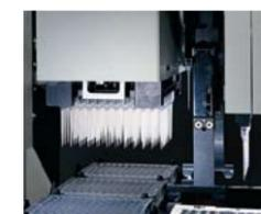
**X/Y/Z carriage configured with four independently moving tools**
