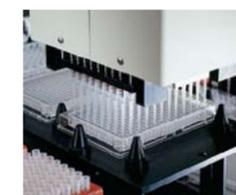
**96-channel pipettor accessing a 384-well microplate**
